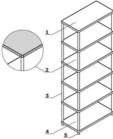
1. **Top** - 19 mm thick varnished MDF board with metal frame (3x30 mm)
